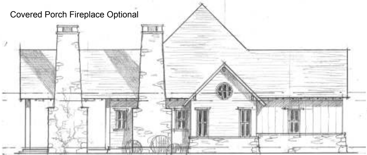
② SETTLEMENT COTTAGE (OPTION #2) LEFT SIDE ELEVATION SCALE: 1/8" = 1'-0"
